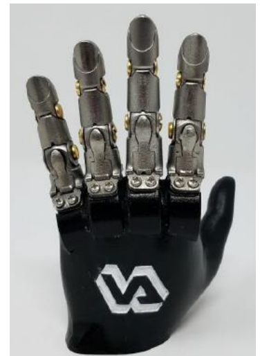
Image: 3D printed women's digits in size suitable for 5 th percentile hands (courtesy of Weir Biomechanics Development Laboratory)
